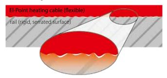
Due to its flexibility, the heating cable can equalise most of the rails irregularities. Thus the **heat transfer into the rail is enhanced** and results in a higher rail temperature at relatively low energy consumption.
