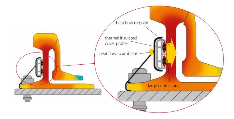
The thermally insulating cover profile reduces heat losses to ambient and directs the heat flow toward the rail. The big, dark rail surface turns into a radiator - the heat radiation frees the gap between stock rail and switchblade effectively from snow and ice. That means: **High** efficiency due to high heat radiation ratio and partial thermal insulation of rail surface by cover profile.
