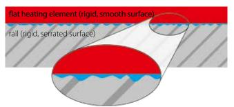
Between the rail and heating element surface, a number of small gaps occur because of the irregularities in the rail surface and the inflexibility of the heating element sheath. The result is a comparatively poor heat transfer into the rail and thus a comparatively low rail temperature.
